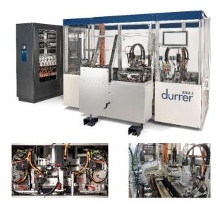
The REGA 3 can handle soft- and hardcover products in the format range up to 350 x 350 mm. All the usual tab shapes can be cut.
