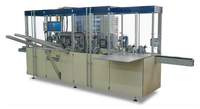
The HANA machine is a automatic machine for processing covers, sticky note pads and film markers. All individual parts are fully automatically assembled to a finished combi-set. The result is a high-quality advertising gift.
