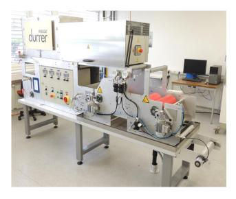
The D300 Web Coater corresponds with the latest technological standards in the industry. The machine enables the coating process to be reproduced very realistically in the laboratory. The comprehensive setting options allow individual formulations to the tested and optimised. The knowledge gained can then be applied on the production machine with high process capability.
