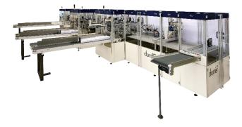
The BLOFIX is a fully automatic processing line to glue blocks on a cardboard or to attach headboards to calendars.
