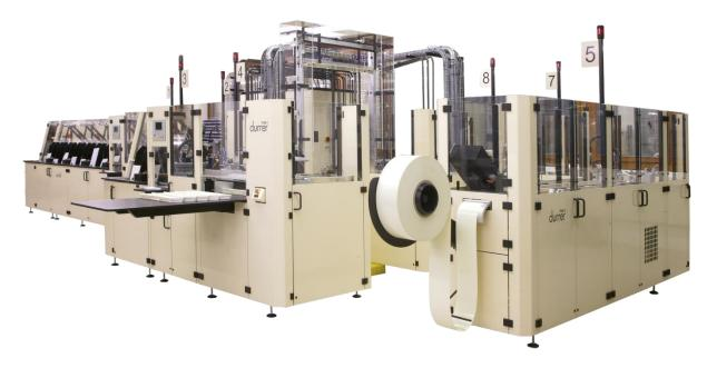
The PLABI 6 makes plastic comb binders, inclusive pre-processing of the book blocks and fully automatic binding of it. The machine consists of several basic modules and can be customized.
