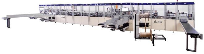
The WIRO 4 is a fully automatic processing line for producing wire bound products inclusive pre-processing of book blocks. The WIRO 4 consists of several basic modules and can be customized. The machine can be put in-line with other machines, e.g. a gathering machine.
